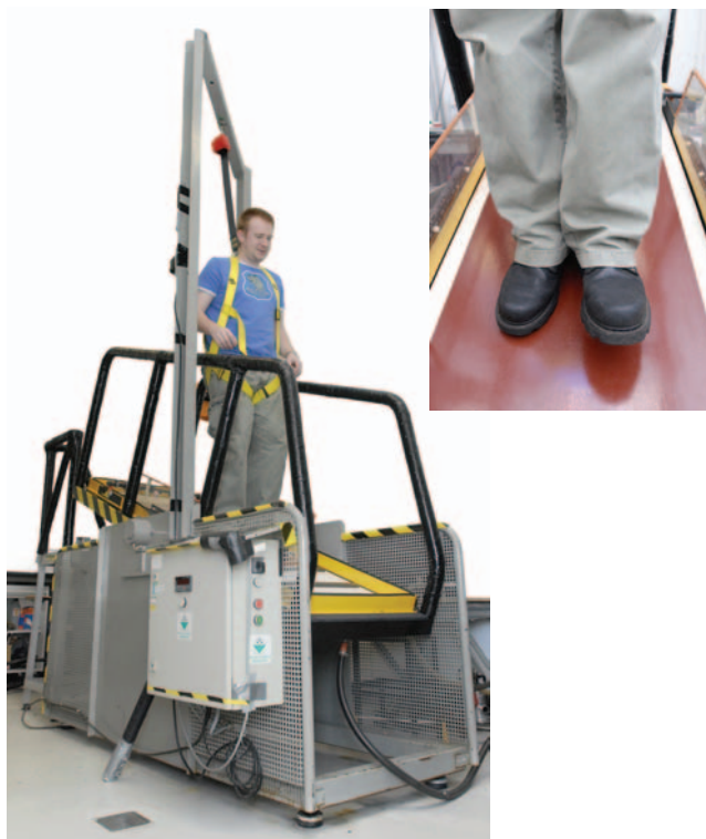
Figure 4 The UKSRG ramp CoF test
